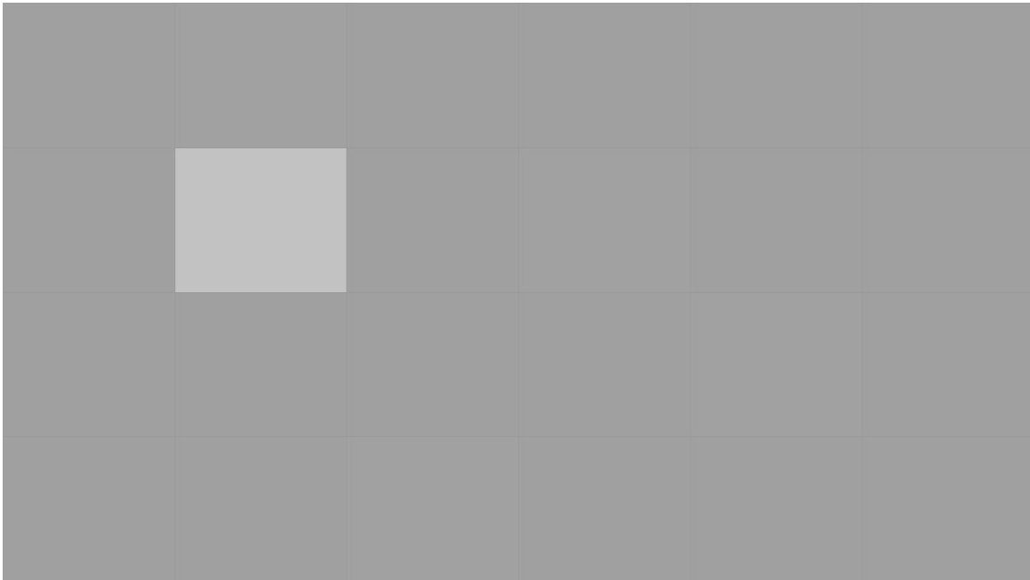
Figure 9-16: Example 1 – Average Code Value 160, Ignore the One Bright (or Dark) Zone Caused by Timing Differences
